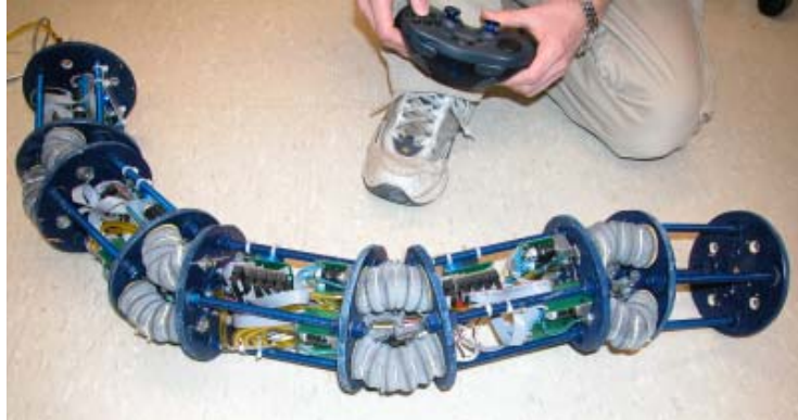
Figure 12: The new OmniTread joints actuation test-bed is made of five dummy segments and four fully functional 2-DOF joints.
