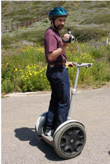
Figure 4: UM researcher Johann Borenstein steadies a camera on a Segway HT platform to obtain preliminary data on motion stability.
