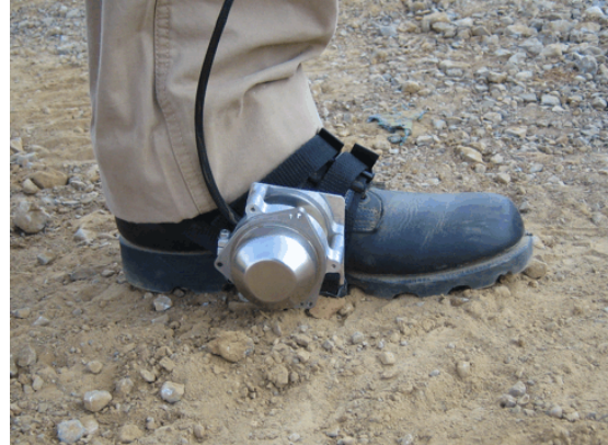
Figure 1: BAE SiIMU02 Inertial Measurement Unit (IMU) mounted to the foot of a walking subject. Of course, this IMU is too large for most practical uses. Our intention is to implement our PDR system with a much smaller IMU in the near future.
