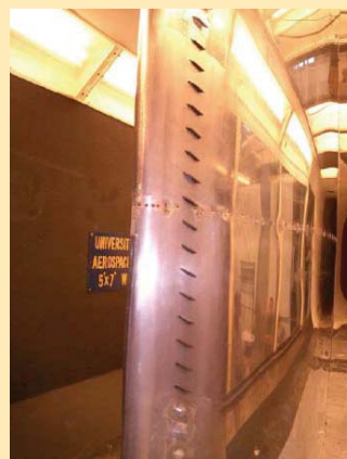
Piezo-compliant actuators embedded in an aircraft wing.
