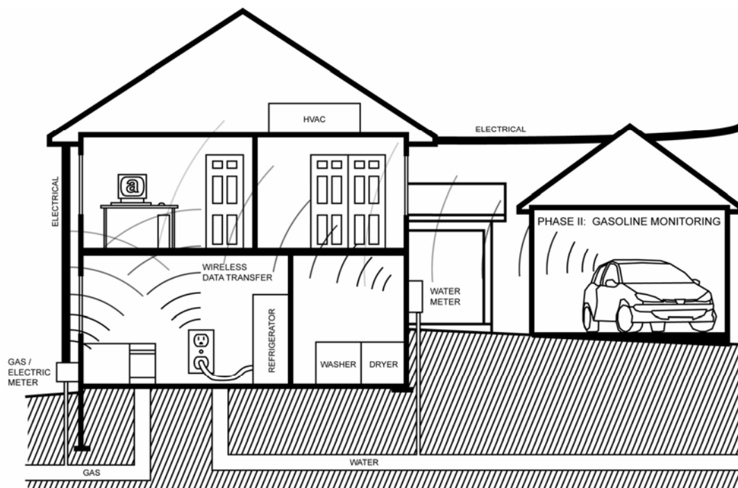
Figure 2. Conceptual illustration of the AWARE@home system. Electronic accumulators and wireless transmitters connect to existing metering technologies (gas, electric, water). A USB-compatible receiver is utilized, along with a device to monitor & transmit electricity consumption of single appliances “plugged in to the wall”.
